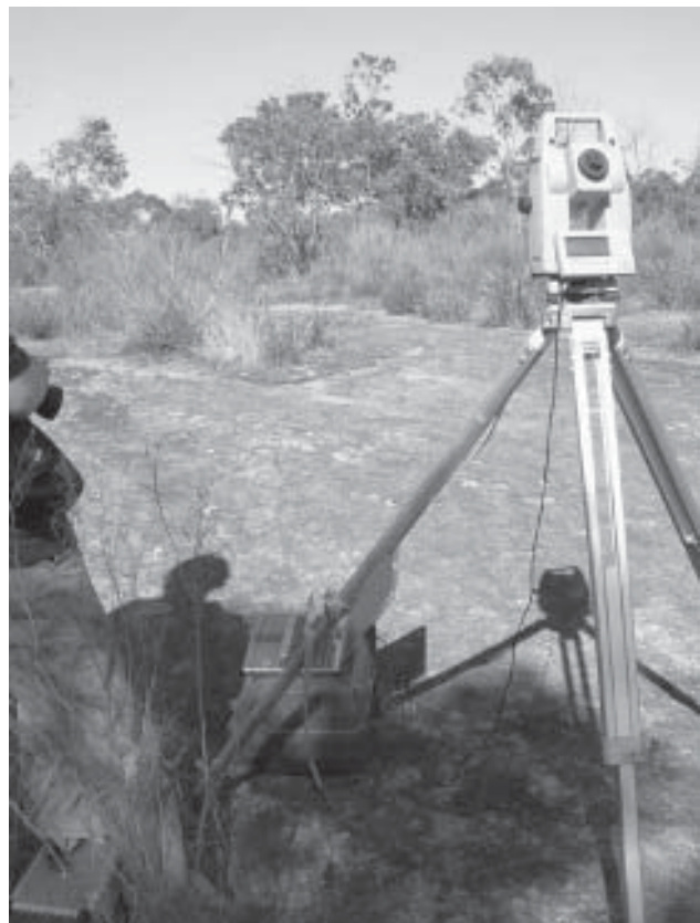
Figure 4. Total Station used for co-ordinating control and generating check data.
