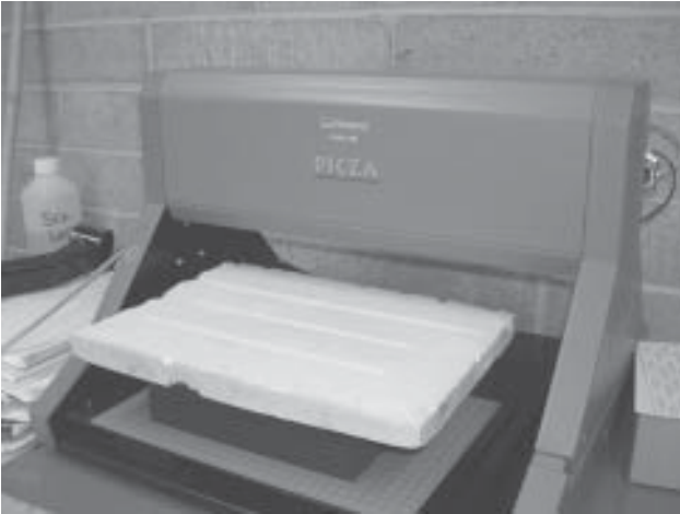
Figure 14. Roland PIX-30 motorised profiler with grooved sandstone slab.
